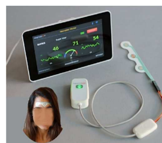
Fig. 1. Neurosteer EEG system. A wearable one-lead medical electrode with a single-use sensor that attaches to the forehead and a relay computer connected to the Neurosteer® Cloud server.
